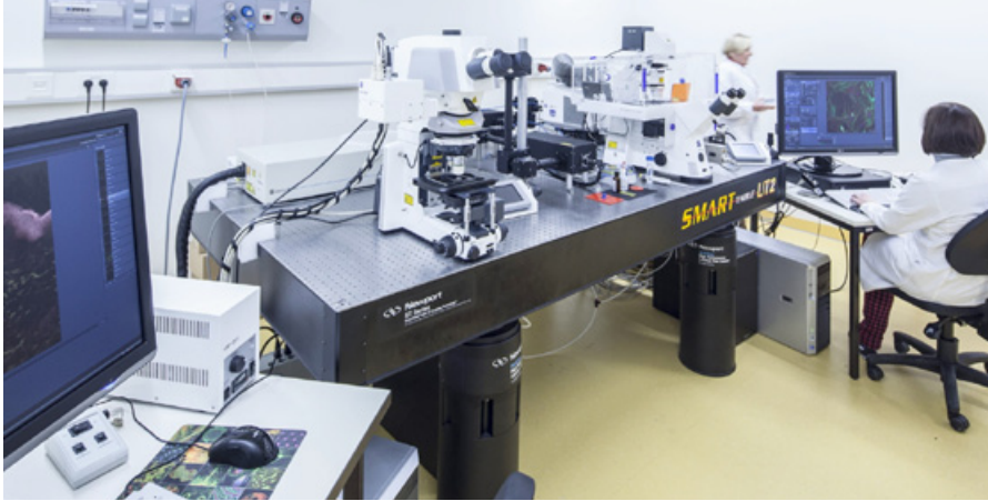
The heart of the core unit: LSM 710 (right); LSM 7 MP (left); and fs-pulsed Ti:Sa laser (middle).
