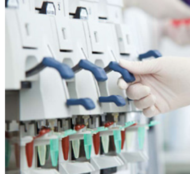
Isolation of murine hematopoietic stem cells via complex multicolor FACS (Fluorescent-Activated Cell Sorting) on a BD FACSAria III cell-sorting machine
